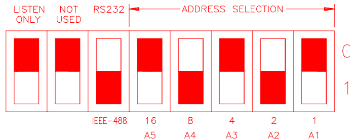
Figure 9-3: GPIB Address Selection Switch
